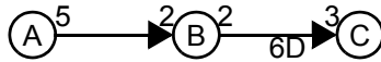
Figure 2. An SDF graph used to illustrate GDPPPO applied to SDF graphs that have nonzero delay on one or more edges. Here \mathbf{q}(A, B, C) = (6, 15, 10) .
