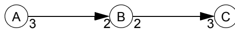
Figure 3. An SDF graph used to illustrate the problem of finding an optimally compact loop structure for an arbitrary firing sequence.
