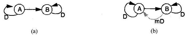
Fig. 2. IPC graph with a feedforward edge. (a) Original graph. (b) Imposing bounded buffers.
