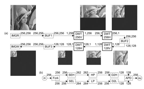
Figure 4.6: A MDSDF graph of two dimensional discrete wavelet transform. (a): 2DSDF graph of 2DDWT, where *DWT256V*, *DWT256H*, *DWT128V*, and *DWT128H* are supernodes for processing 1-D DWT for 256-pixel/128-pixel columns/rows. (b): 1DSDF subgraph of *DWT256V* and *DWT256H*.
