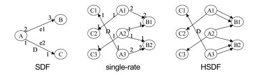
Figure 2.1: Conversion between SDF, single-rate, and HSDF.
