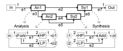
Figure 4.2: Hierarchical SDF graphs of a tree-structured filter bank. (Supernodes are shown in bold blocks; and production and consumption rates are indicated at the ends of edges and alongside ports.)
