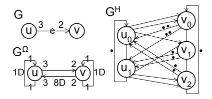
Figure 8.1: SDF graph G,  $\Omega$ -SDF graph  $G^{\Omega}$  given buf(e) = 8, and the transformed  $\Omega$ -HSDF graph  $G^{H}$ .
