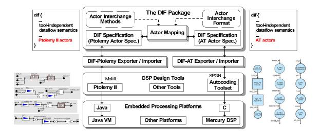
Figure 5.2: The DIF-based porting mechanism.
