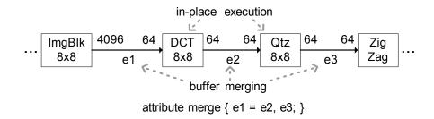
Figure 6.4: An in-place buffer merging example in JPEG.
