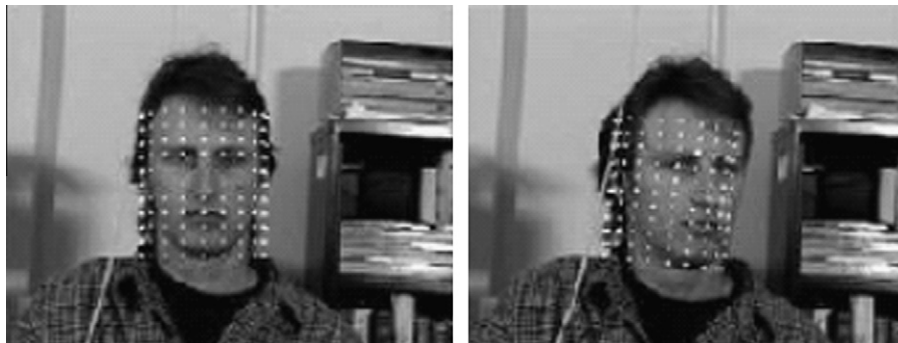
Fig. 5. An example of 3D facial pose tracking with a cylindrical mesh.
